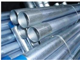
They may be joined easily, threading, cutting, and bending them is also an easy task. They are joined with the help of a socket. These pipes are light-weighted and cheap. Acidic and alkaline waters affect these pipes badly.
